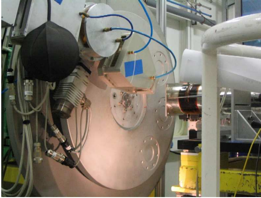
Figure 2.11: A picture of the powder diffractometer at the beam-line ID31.
